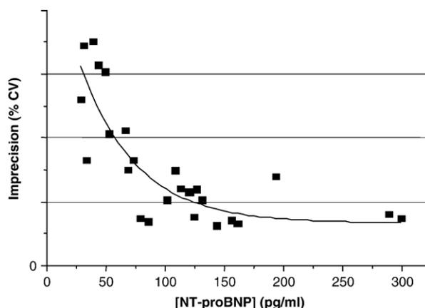
Fig. 1. Functional sensitivity of the RAMP NT-proBNP assay: functional sensitivity=57 ng/L at 20% CV. CV: Coefficient of variation.
